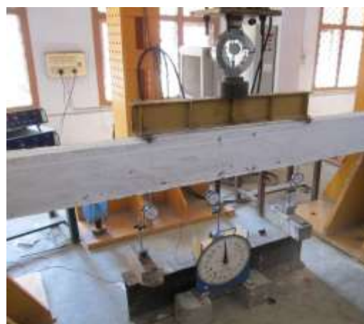
Fig.3 Testing of RC Beam in the laboratory
