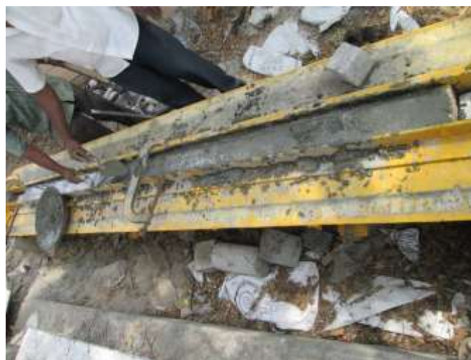
Fig 2 Casting of Reinforced concrete beam in the laboratory
