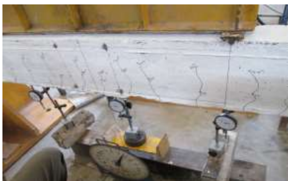
Fig.5 Crack Pattern of RC Beam
