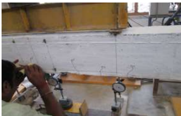
Fig.4 First Crack of RC Beam
